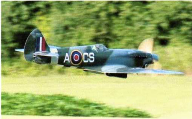
Despite its thin and pointed wingtips, Dave Szabo's Spitfire has excellent handling due, in part, to about 2 1/2 degrees of washout, slightly more than the full-sized Spit. Low pass before a chandelle shown here.
