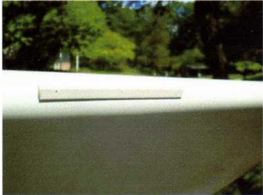
A 90-degree sharp edge stall strip is added to the leading edge of the Grumman Lynx leading edge to lower the stall angle in the root area of the wing. This alternative to washout works when inverted too.
