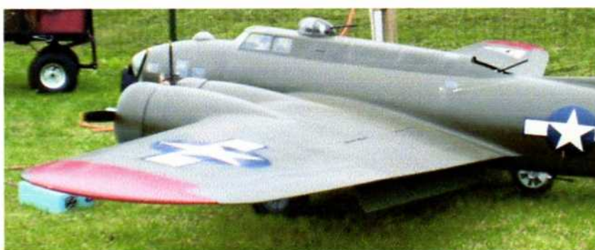
Washout provides good yaw control in Greg Hahn's B-17 in case of engine failure.
