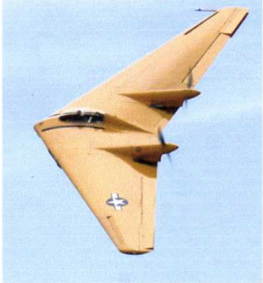
The Northrup N9M flying wing depends upon sweep-back and washout for all of its pitch stability. Note the leading-edge slats for an extra margin of stall control at the tips.
