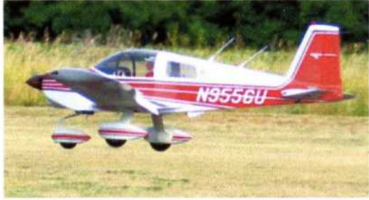
A 90-degree sharp edge stall strip is added to the leading edge of the Grumman Lynx leading edge to lower the stall angle in the root area of the wing. This alternative to washout works when inverted too.
