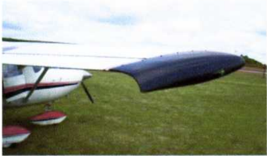
Bob Patton's Cessna Aerobat uses drooped wingtips for stall control, typical of Short Take-Off and Landing (STOL) aircraft.
