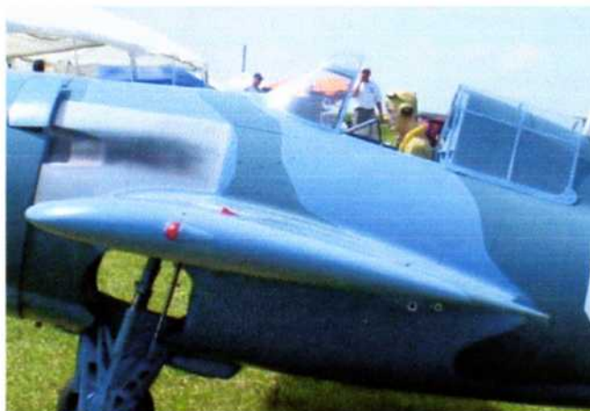
No washout and no incidence in Dave Deschenes' Wildcat, also typical of nearly constant-chord dive bombers.
